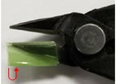
A close-up photograph of the pliers with the green tape covering the front and interior. The remaining part of the tape is being folded over the outer edge of the blade. A red arrow indicates the direction of the fold.                | <p>Pliez le reste du ruban adhésif sur l'extérieur de la lame.</p>                                                                                                                                            |
