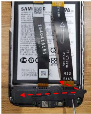
A close-up photograph of the bottom part of the smartphone. A black speaker cover is being placed diagonally over the charging port area. Red arrows indicate the diagonal placement and the bottom edge being aligned.                              | Placez la partie inférieure du boîtier du haut-parleur en diagonale sur le connecteur de charge et assemblez la partie supérieure. |
