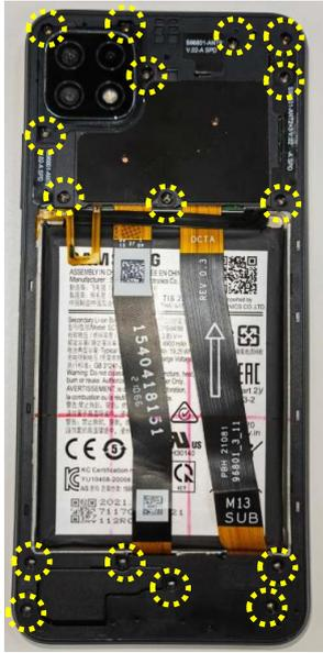
A photograph of the back of the smartphone with the back cover and speaker cover in place. 16 screws are highlighted with yellow dashed circles, indicating where they should be tightened.                                                         | Serrer les 16 vis                                                                                                                  |
