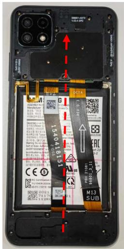
A photograph of the back of a Samsung smartphone with the back cover removed. The main board is visible. A black back cover is being positioned diagonally over the board. Red arrows indicate the diagonal placement and the top edge being aligned. | Positionnez la surface inférieure du cache arrière en diagonale sur la carte mère principale et assemblez la surface supérieure.   |
